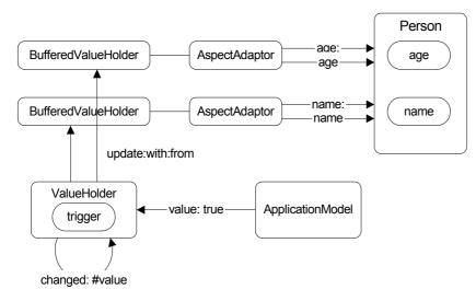
Figure 24-6. The BufferedValueHolder mechanism.
